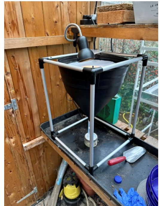
Fig. 1. Berlese Funnel set up in the greenhouse.
