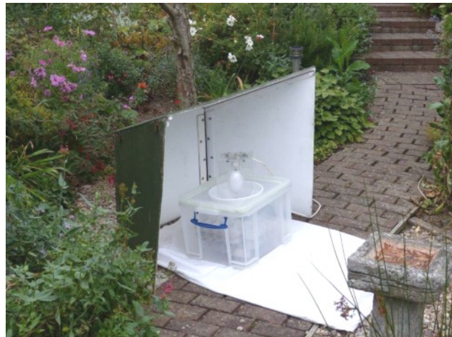
Our mercury vapour moth trap was made by Adrian Russell. We added the shroud at the back to avoid dazzling our neighbours.
